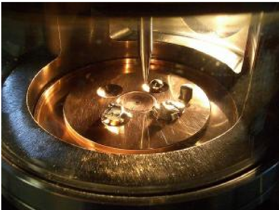
Arc melter in which a plasma of up to 3000°C is produced between a tungsten tip (center) and a water-cooled copper plate. (Credit: ETH Zurich/LMPT)
