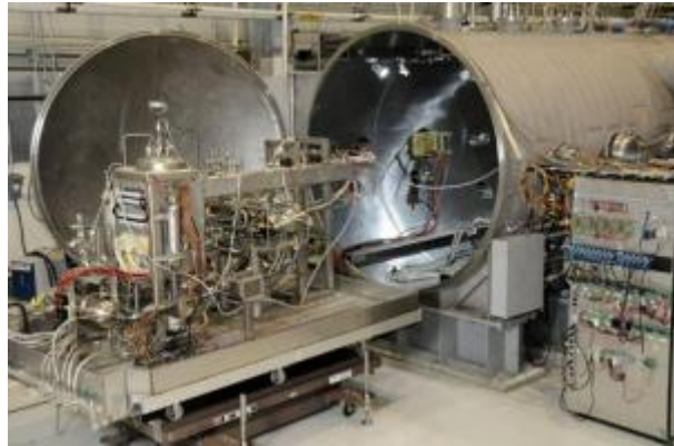
The Stirling engine test configuration upon removal from the vacuum chamber. (Credit: NASA/MSFC/E. Given)
